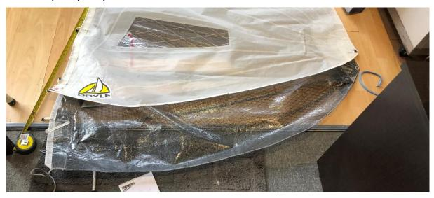
Headsail foot median for standard headsails varies from 3760mm to 3785mm
